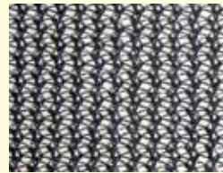
WS70BK* 1/8" Knitted Polyethylene Opacity 70 %
